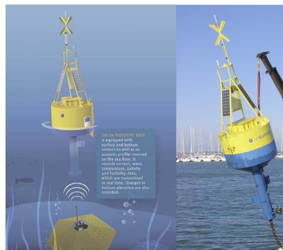
Figure 10: Schematic view of the Previmer-D4 platform (left) and a photograph of the real buoy (right).
